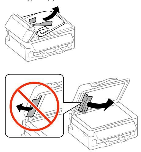
**Caution:** Do not remove paper jammed inside the ADF without opening the cover or you could damage the ADF.
